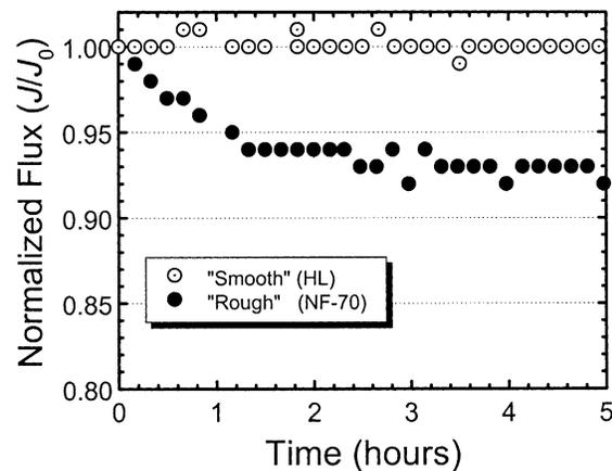
Fig. 7. Experimental flux decline (fouling) data comparing “smooth” HL and “rough” NF-70 nanofiltration membranes. Test conditions employed were: initial flux ( $J_0$ ) =  $1.415 \times 10^{-5}$  m/s (30 gfd), feed particle concentration ( $C_p$ ) = 200 mg/l (0.009% (v/v)), ionic strength ( $I$ ) = 10 mM NaCl, crossflow velocity ( $u_{XF}$ ) = 0.192 m/s, shear rate ( $\gamma_0$ ) =  $1334 \text{ s}^{-1}$ , temperature =  $25^\circ\text{C}$ , and pH =  $6.8 \pm 0.2$ .
