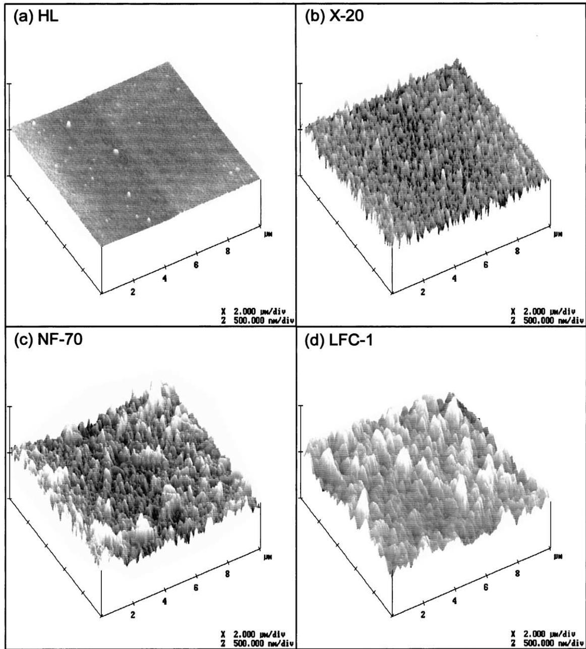
Fig. 3. AFM images of (a) Osmonics HL (NF); (b) Trisep X-20 (RO); (c) Dow-FilmTec NF-70 (NF); (d) Hydranautics LFC-1 (RO) membranes. Note that the X and Y dimensions are both  $10\ \mu\text{m}$  ( $2\ \mu\text{m}/\text{division}$ ), while the Z-scale is  $1\ \mu\text{m}$  ( $500\ \text{nm}/\text{division}$ ). Average roughness parameters calculated for each membrane were 10.1, 33.4, 43.3, and 52.0 nm for HL, X-20, NF-70, and LFC-1, respectively.
