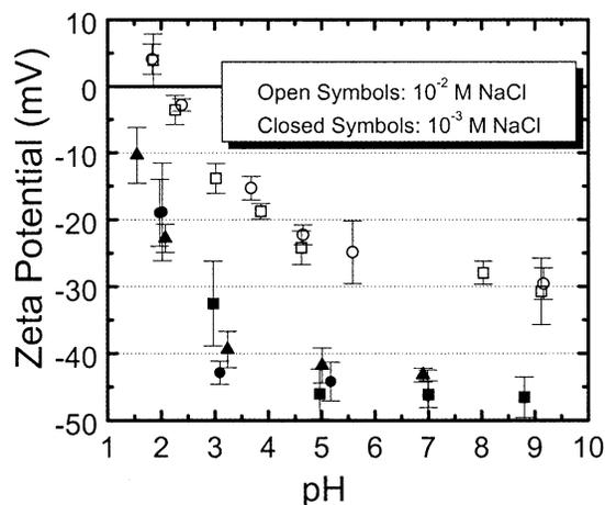
Fig. 6. Zeta potential behavior of the model silica colloids as a function of pH for ionic strengths of 1 mM NaCl (closed symbols) and 10 mM NaCl (open symbols). At the test conditions employed in most fouling experiments (0.01 M NaCl and pH  $6.8 \pm 0.2$ ) the zeta potential of the model colloids was approximately  $-25$  mV.
