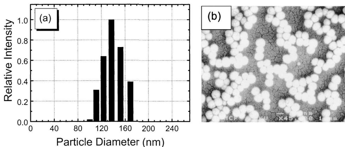
Fig. 5. Particle size and shape analysis from (a) dynamic light scattering measurements; (b) scanning electron microscopy.
