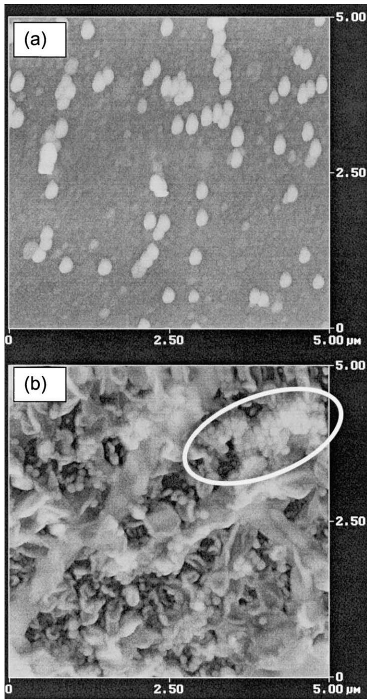
Fig. 8. Tapping mode AFM images of (a) HL, and (b) NF-70 nanofiltration membranes. Fouling test lasted for 30 s and test conditions were: initial flux ( $J_0$ ) =  $1.415 \times 10^{-5}$  m/s (30 gfd), feed particle concentration ( $C_p$ ) = 20 mg/l (0.0009% (v/v)), ionic strength ( $I$ ) = 10 mM NaCl, crossflow velocity ( $u_{XF}$ ) = 0.192 m/s, shear rate ( $\gamma_0$ ) =  $1334 \text{ s}^{-1}$ , temperature =  $25^\circ\text{C}$ , and pH =  $6.8 \pm 0.2$ .
