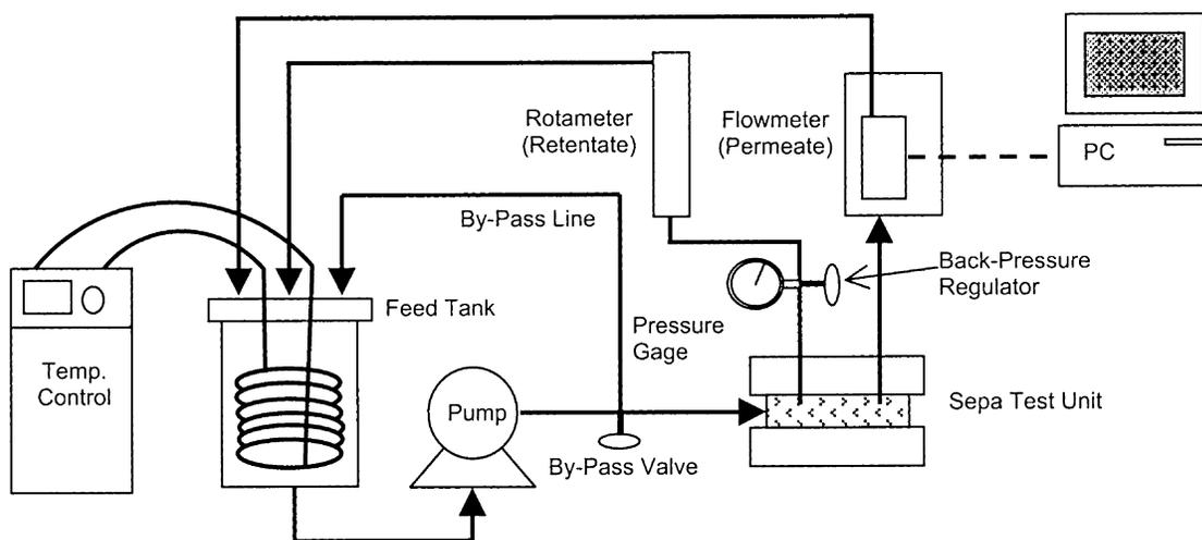
Fig. 1. Modified "Sepa CF" recirculating crossflow membrane-filtration apparatus used in colloidal fouling experiments.
