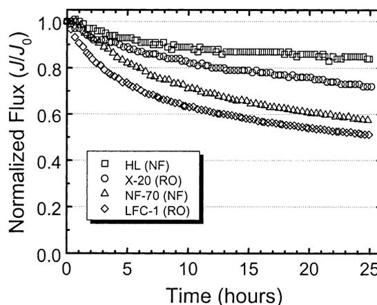
Fig. 2. Experimental flux decline (fouling) data for Osmonics HL (NF), Trisep X-20 (RO), Dow-FilmTec NF-70 (NF), and Hydranautics LFC-1 (RO) membranes. Test conditions employed were: initial flux ( $J_0$ ) =  $1.415 \times 10^{-5}$  m/s (30 gfd), feed particle concentration ( $C_p$ ) = 200 mg/l (0.009% (v/v)), ionic strength ( $I$ ) = 50 mM NaCl, crossflow velocity ( $u_{XF}$ ) = 0.096 m/s, shear rate ( $\gamma_0$ ) =  $324 \text{ s}^{-1}$ , temperature = 25°C, and pH =  $6.8 \pm 0.2$ .
