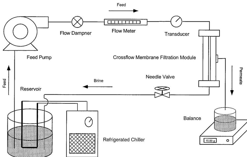
FIG. 2. Schematic description of the laboratory-scale crossflow membrane filtration unit.
