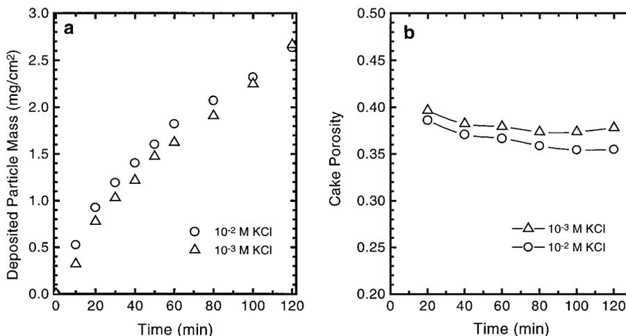
**FIG. 8.** Change of (a) particle accumulated mass and (b) cake layer porosity for crossflow experiments with the 100 nm particle suspension. Filtration conditions employed were: temperature, 20°C; particle volume concentration, 0.01% ( $1.91 \times 10^{17} \text{ m}^{-3}$ ); transmembrane pressure, 41.4 k Pa; and shear rate,  $280 \text{ s}^{-1}$  (or crossflow velocity, 0.246 m/s). Filtration experiments were carried out at pH 10 and  $10^{-2}$  M KCl.
