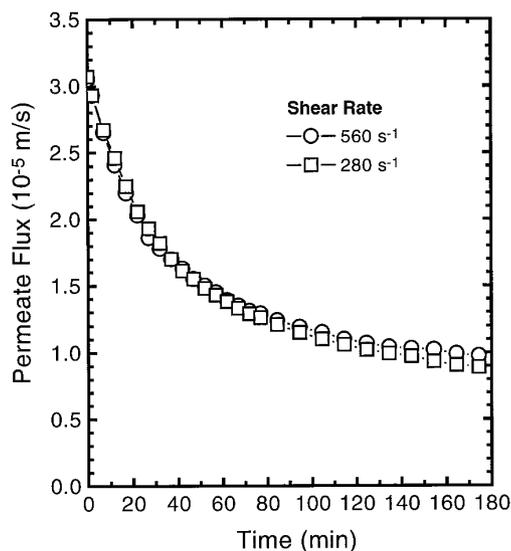
**FIG. 6.** Effect of shear (crossflow) rate on permeate flux decline in crossflow filtration with the 100 nm silica suspension. Filtration conditions employed were: temperature, 20°C; particle volume concentration, 0.01% ( $1.91 \times 10^{17} \text{ m}^{-3}$ ); and transmembrane pressure, 41.4 k Pa. Filtration experiments were carried out at pH 10 and  $10^{-2} \text{ M}$  KCl.
